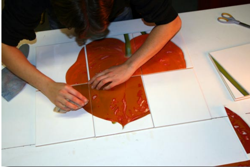
Manufacture of a shower room decoration - application and alignment of the transfer/decals to the tiles before drying & firing
